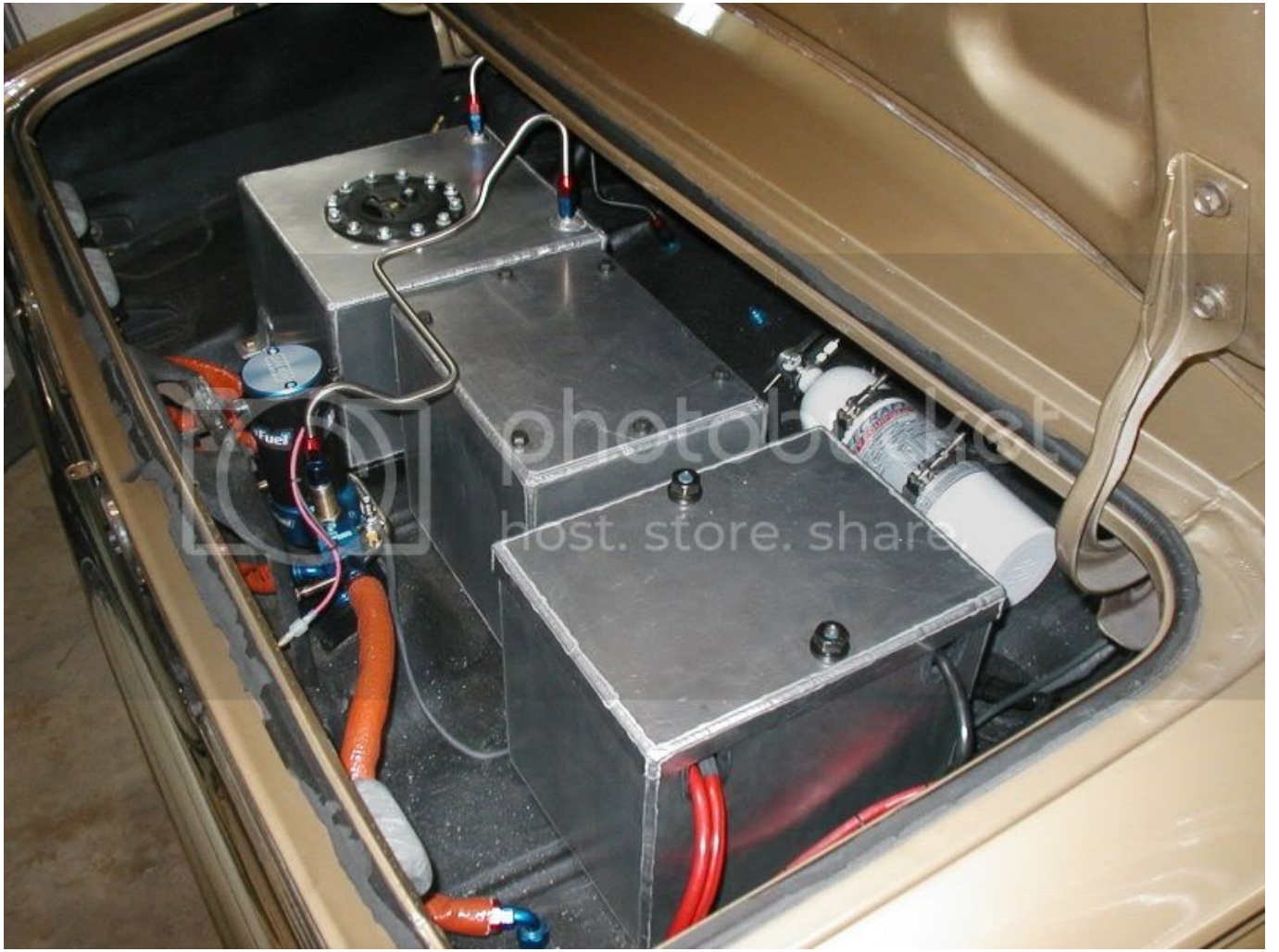
Magnafuel Prostar 500 Installation
